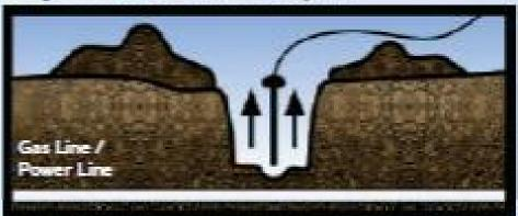
Only oscillating head type noticles are to be used for the water wand. When excavating within 1 metre horizontally of a marked line the maximum settings of 38°C water temperature and 10.340 Kpa (1,500 psi) must not be exceeded. The end of the vacuum tube shall be neoprene or equivalent. Expose the buried line by using a SWEEPING MOTION ONLY, perpendicular to the locate markings, until the line is sighted. After sighting, the line shall not be contacted by spray or vacuum.
