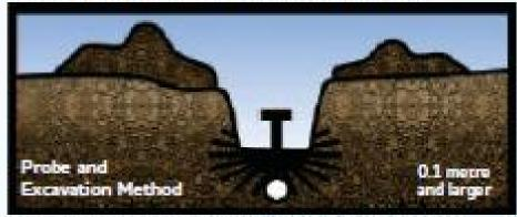
In addition to other excavation methods previously mentioned, a probe and excavate technique can be used for gas pipelines 0.1 metro and larger in diameter.
