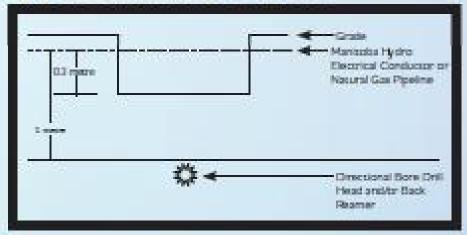
Drilling below a Manitoba Hydro electrical conductor or natural gas pipeline.
